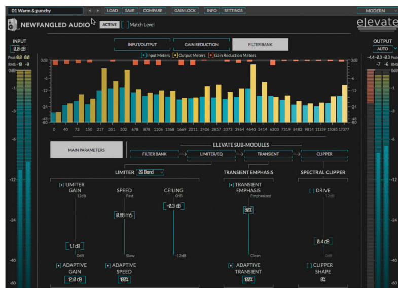
Fig. 1: Elevate's Main Parameters view shows key controls for the Limiter, Transient Emphasis and Spectral Clipper processing blocks.
