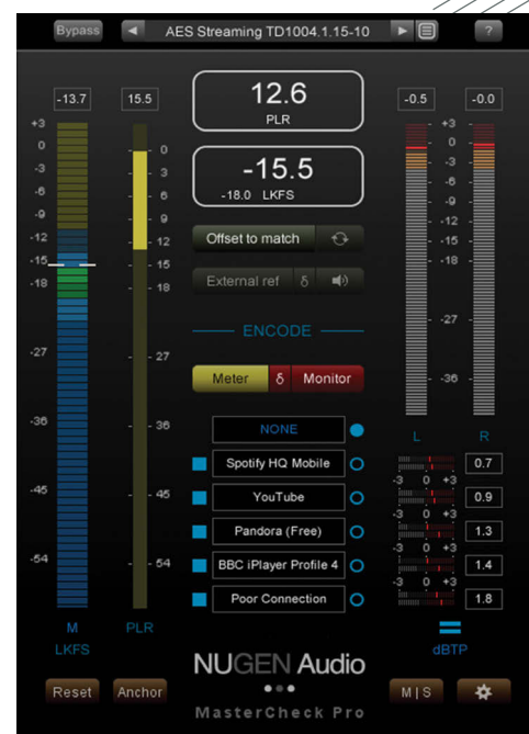
MasterCheck Pro allows real-time encoding and auditioning of lossy data compression algorithms used by different services.
