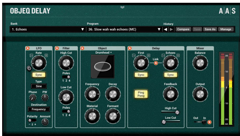
Objeq Delay's input signal excites one of four virtual objects before going on to two delays chained in series. More than a dozen parameters can be modulated using a variety of editable LFO waveforms.
